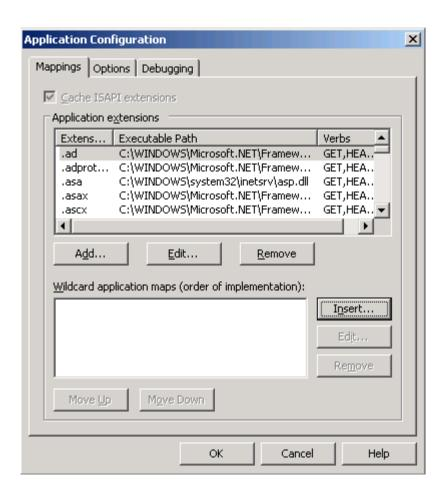
b) On the Mappings tab, click the "Insert..." button next to the "Wildcard application maps" area. Select the file aspnet\_isapi.dll. On a 32-bit OS, the path will be "\WINDOWS\Microsoft.NET\Framework\v2.0.50727\aspnet\_isapi.dll". On a 64-bit OS, the path will be
