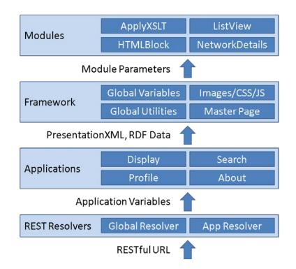
Modules typically obtain data by performing an HTTP POST to a URI that returns an RDF document. That URI can exist anywhere on the internet. If the URI happens to be in Profiles, then the HTTP POST will pass through the REST Resolver and be handled by the Profile application. Thus, the Display application usually calls the Profile application multiple times indirectly via the Modules that it tells the Framework to render.
